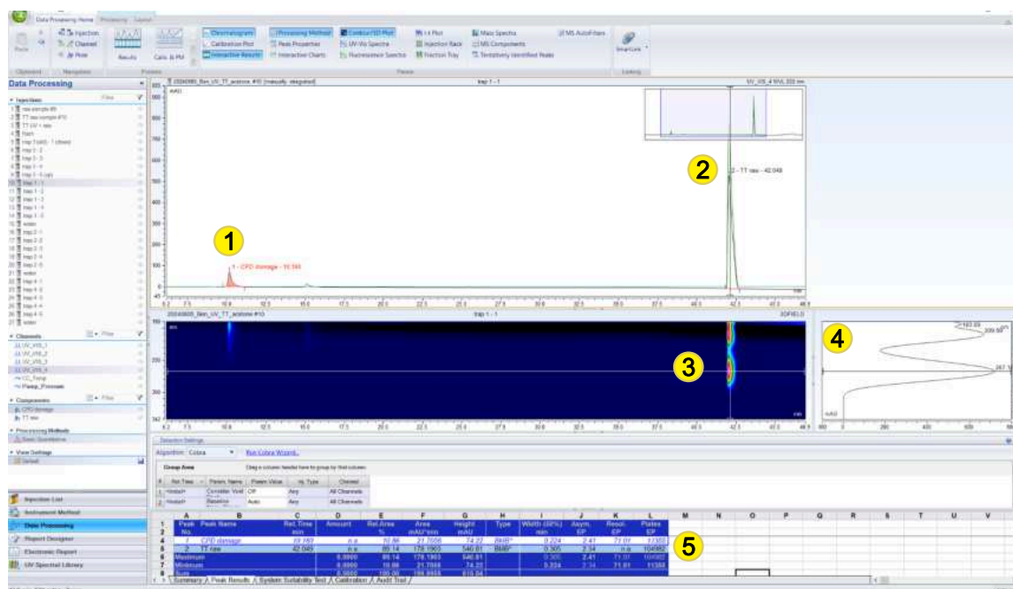
Fig. 20: Chromeleon: screenshot of data analysis. Yellow markers: (1): area computation of peak; (2): specification of time for data output; (3): contour plot of detection signal; (4): absorption spectrum at specific time; (5): numerical output of predefined data points
