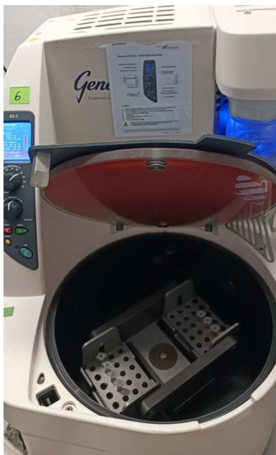
(a) Freeze-evaporator Genevac EZ-2
